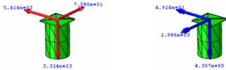
Figure 51. Force and Moment components for base of interior Column 2B under seismic loading.
