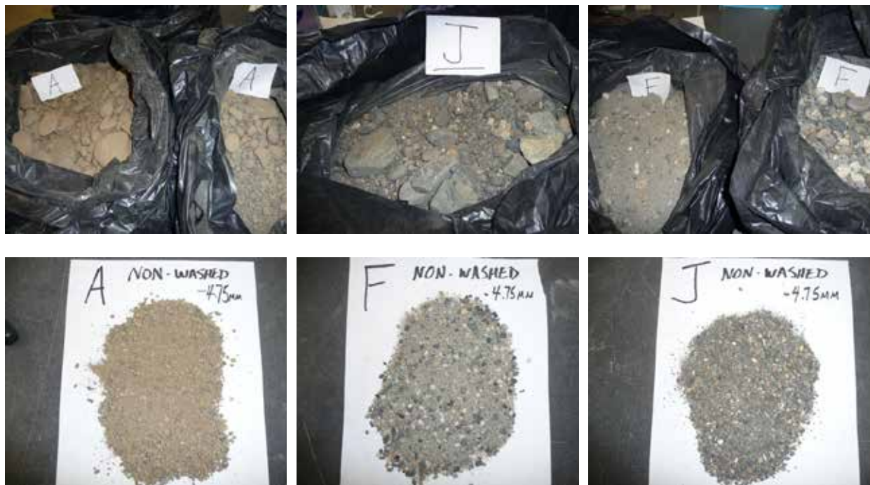
Figure1. Photographic documentation of the aggregate; top: in as-received condition, bottom: after sieving to eliminate fraction larger than 4.75mm
