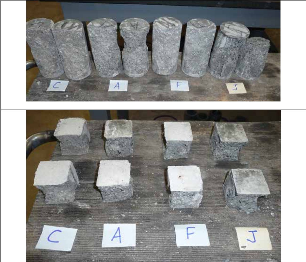
Figure 4. Photographic documentation of samples after failure at 7 days
