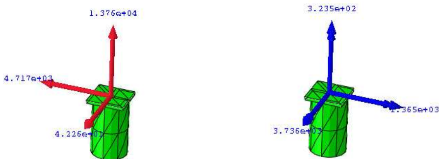
Figure 45. Force and Moment components for base of exterior Column 4A under seismic loading.
