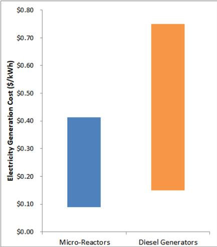
Micro-reactors provide a combination of benefits not provided by other energy sources—they are highly resilient, carbon-free, flexible, and can produce electricity on demand and can operate for years without the need to refuel. In comparison, diesel generators rely on an off-site supply and on-site storage of large amounts of diesel fuel, the delivery of diesel fuel is subject to weather-related interruptions, and they also emit carbon dioxide, particulate matter, and other air pollutants.
